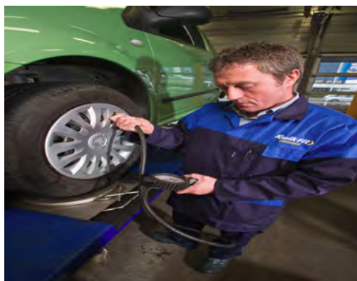
Measuring the pressure inside a tyre using a pressure gauge.
