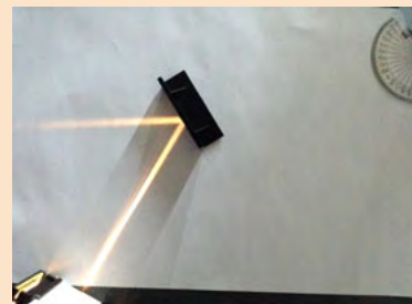
A mirror is placed on the line and a ray is shone to strike the mirror at the normal line.
